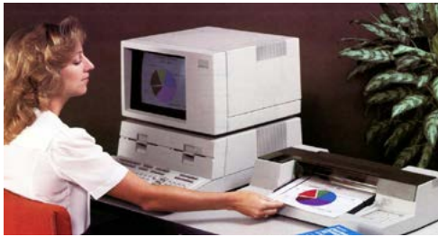
The HP 7475A (1984) with 6 pen carousel in action.
