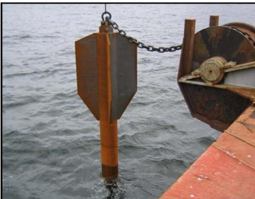
Anchor under deployment showing chain connection
