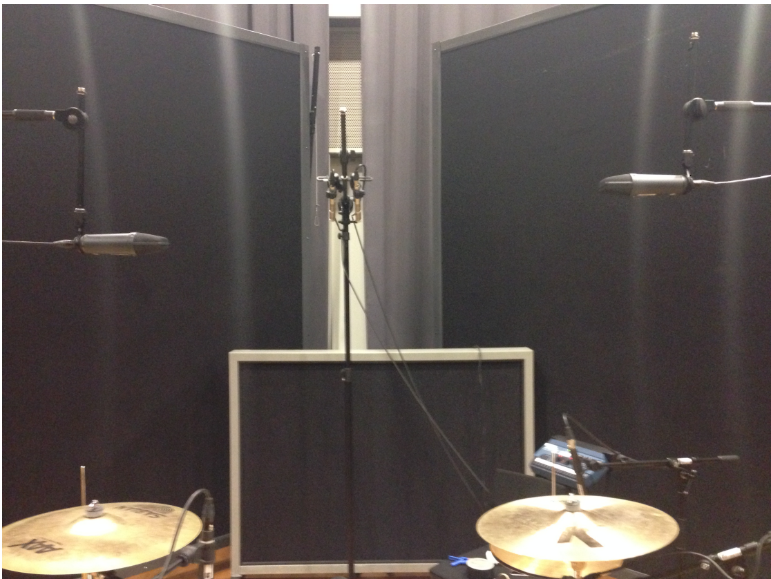
figure 03 - the Audio-Technica AT4081 ribbon microphones placed over the drummer's head
