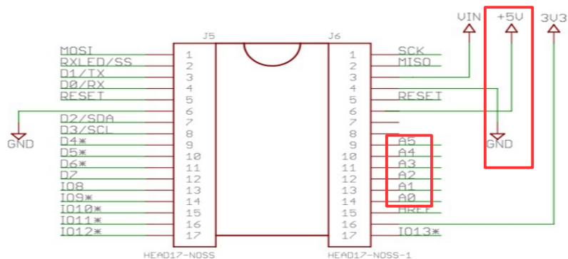
Illustration 12: Diagram of Arduino micro's connections. Ground, power, and used input pins highlighted
