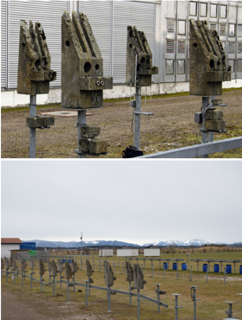
Image 3. Large outdoor stone exposure trials like the Asterixe at the Fraunhofer Institute in Holzkirchen, Bavaria, Germany. Photographs courtesy of Katrin Wilhelm.
