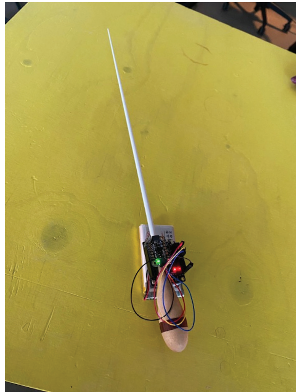
Fig. 2. Conducting baton with accelerometer, microcontroller, and LiPo Battery. (© Majella Clarke)
