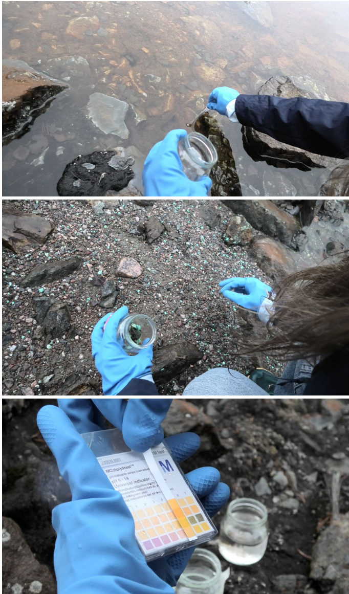
Fig.5-7. Sample collection and pH measurements conducted at Orijärvi Mine. Images courtesy of Camille van Hoffelen.
