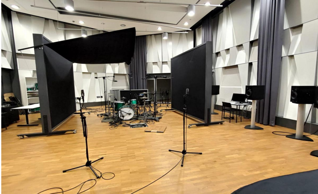
Image showing two C414 microphones to capture the room in stereo
