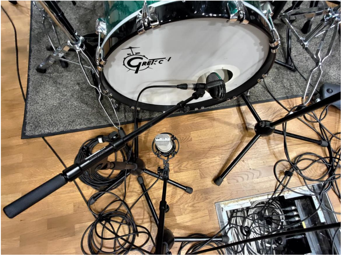
Image from the drum recording session at big recording room, Sibelius Academy, Helsinki. Featuring: Dynamic microphone close to the drum to capture the hard kick drum hit, a condenser microphone placed a little bit away from the kick drum to capture the whole sound.
