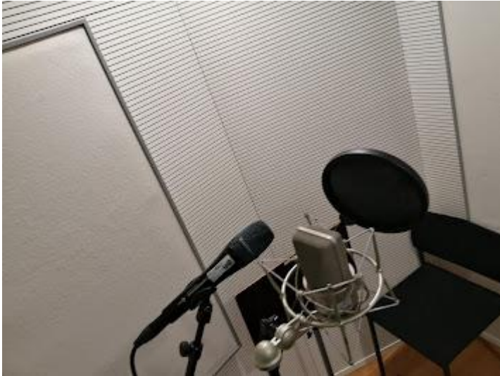
Image of Sennheiser e965 and Neumann TLM 102 Microphone placement for the vocal recording of 'oh Mama, Mama'
