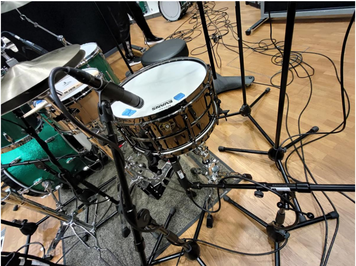
Snare drum with Shure SM 57 Microphone placement on the side
