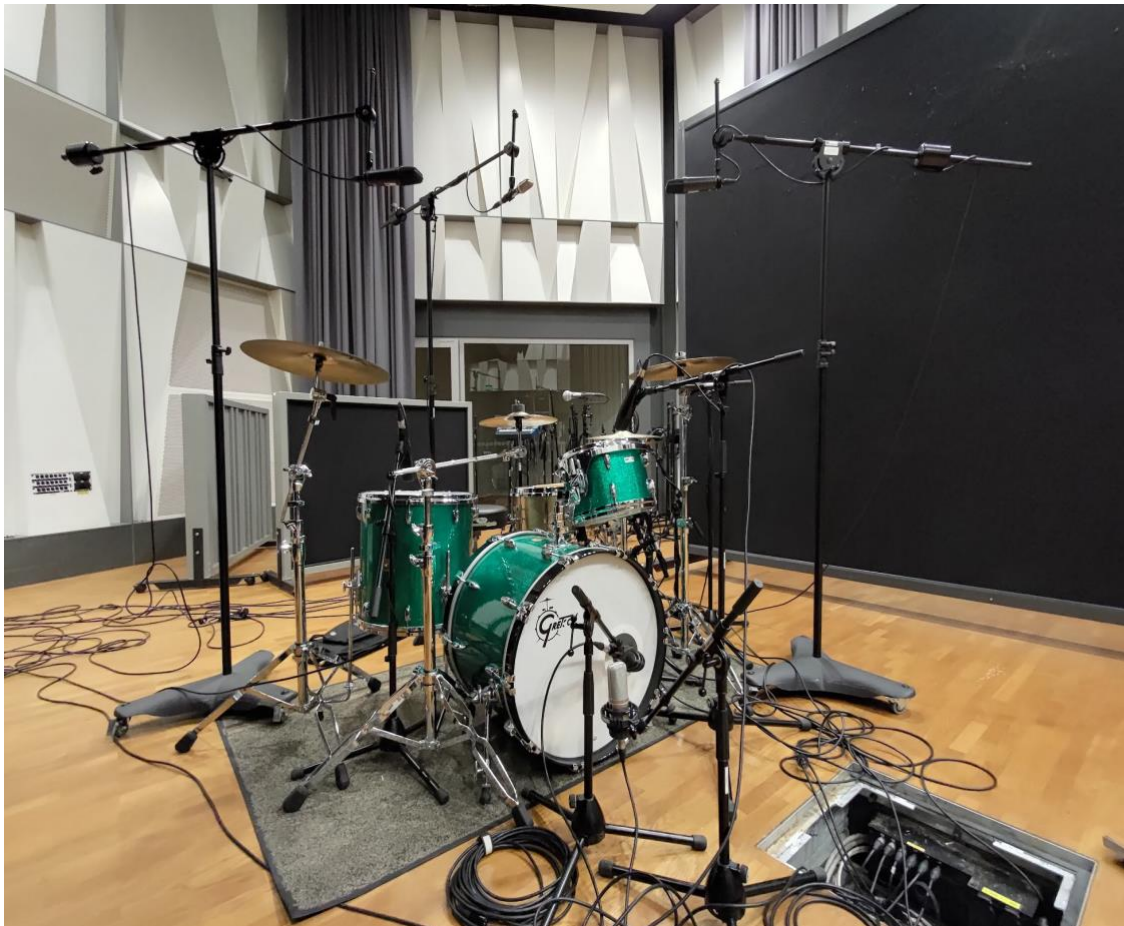
Two Neumann U87 microphones positioned to capture the overhead sound in stereo
